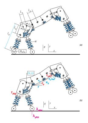
Figure 1: In this work we explore the energetic effects of various spine morphologies on a robotic quadrupedal model. This figure shows the system parameters (a) and generalized torques and coordinates (b) for a 4-segment model. This work will explore models ranging from one to six-segments.
